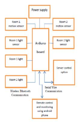
Fig 4: Block diagram of Intelligent Lighting System
