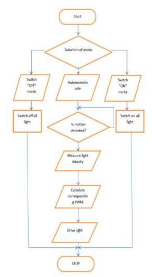
Fig 3: Flowchart of Intelligent Lighting control algorithm
